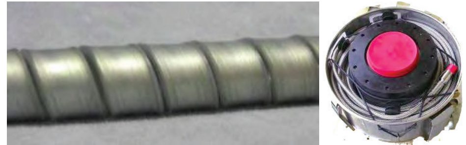
LDPE encapsulated tin lead tape on left. Flex Hose assembly on right.
