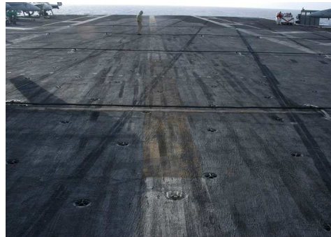
Figure 3: TRI/Austin's Tough-Grip™ non-skid coating deployed aboard the USS Truman.
